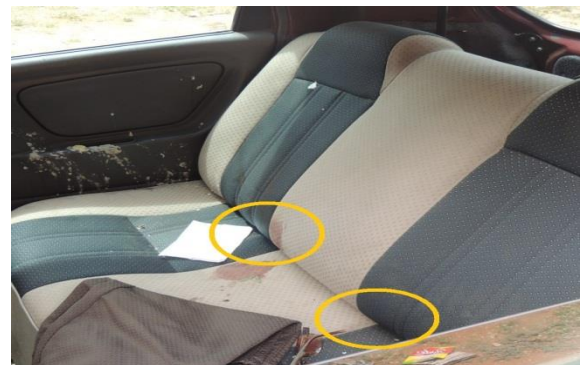
Again, hidden seat buckles made the seat belts unavailable for use.
