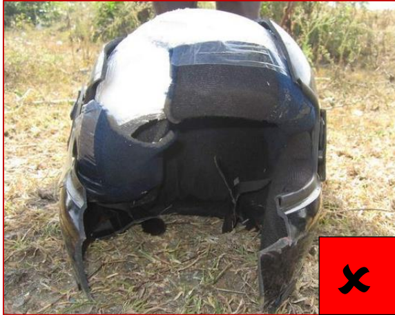
Damaged helmets were found in few Coimbatore crashes indicating the use of sub-standard quality helmets.
