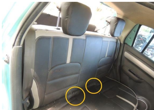
Although seat belts are present, people consider the buckles a hindrance—so they push the buckles behind the seats.
